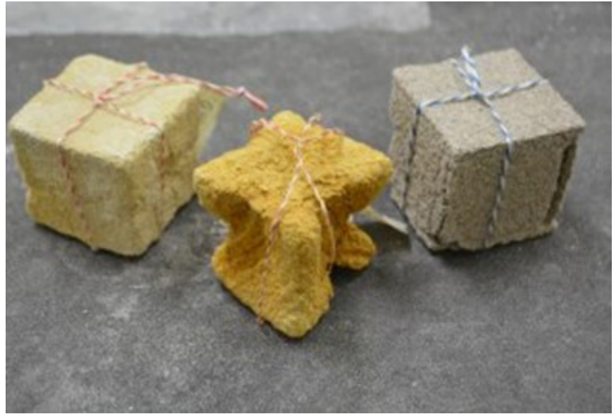
Cubes of stone after resistance to salt attack testing. The stone in the centre has failed and is not considered durable.
